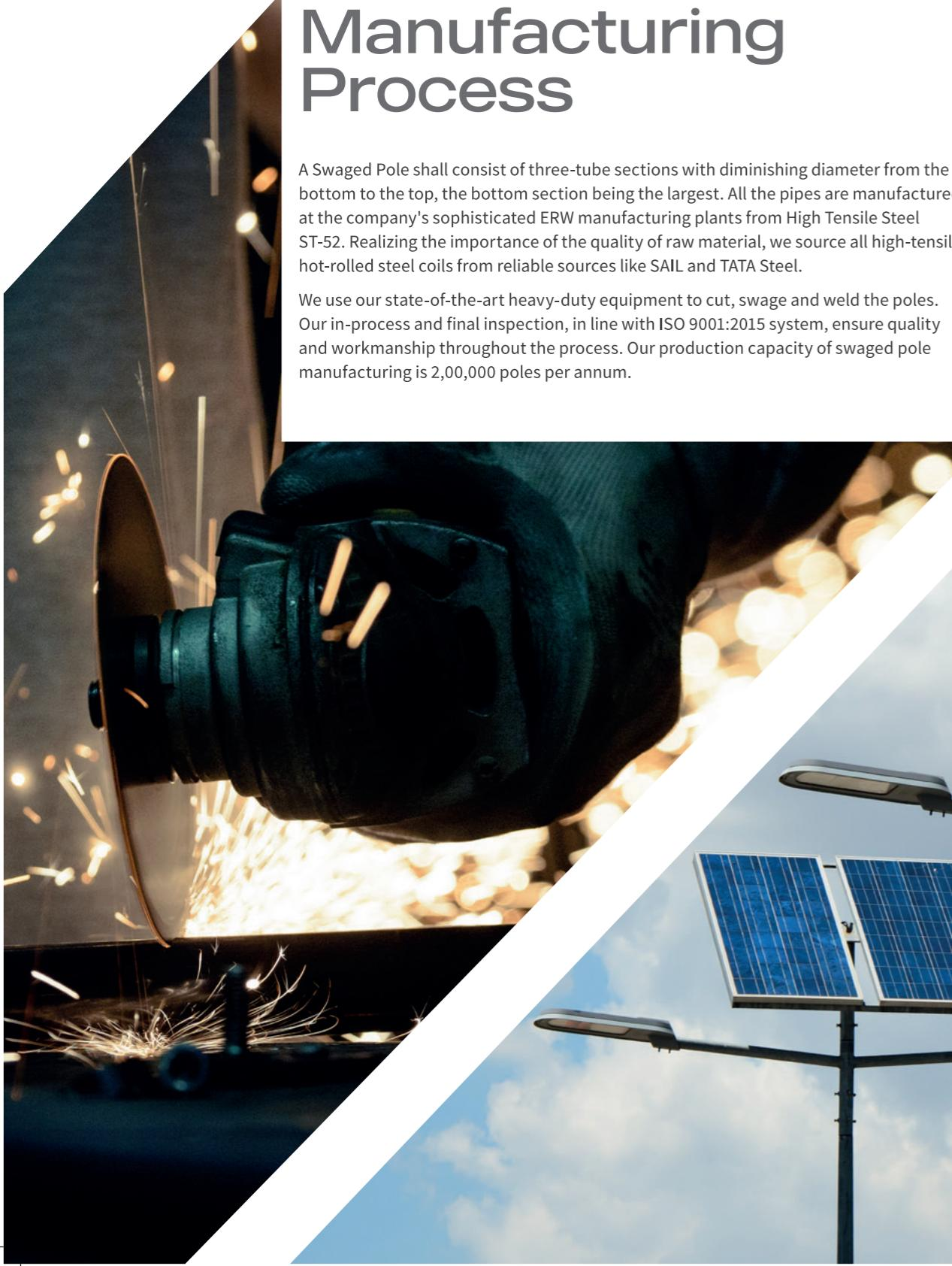
A Swaged Pole shall consist of three-tube sections with diminishing diameter from the bottom to the top, the bottom section being the largest. All the pipes are manufactured at the company's sophisticated ERW manufacturing plants from High Tensile Steel ST-52. Realizing the importance of the quality of raw material, we source all high-tensile hot-rolled steel coils from reliable sources like SAIL and TATA Steel.
